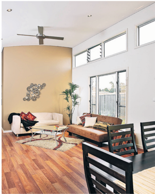
The high-set louvre windows in the living area provide plenty of light and good cross-flow.
